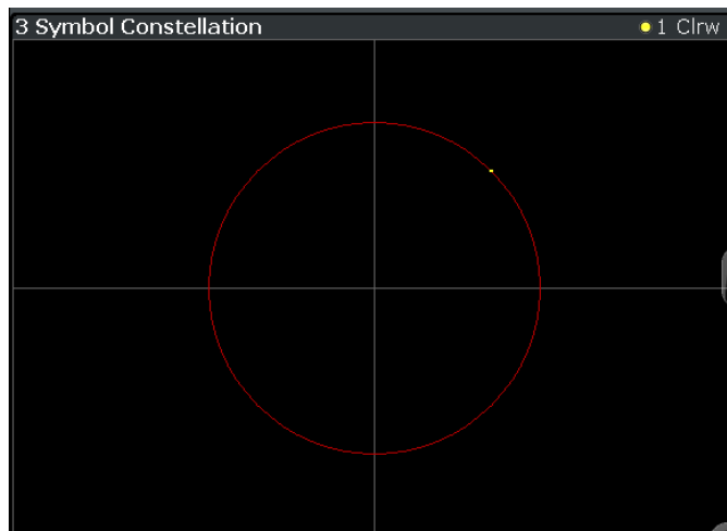
Fig. 3-16: Symbol Constellation display for 3GPP FDD BTS measurements
