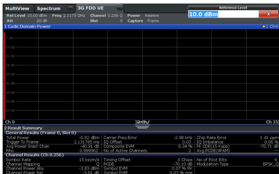
Fig. 10-3: Measurement Example 3: Measuring the Relative Code Domain Power
